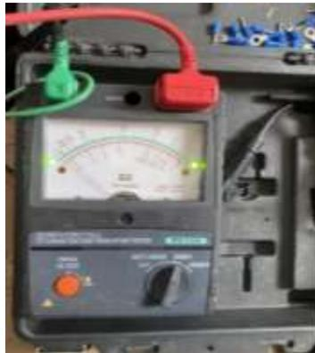
Gambar 3. Alat Ukur Megger *Type Kyoritsu 3123A*
