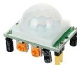
■ Gambar 8. Sensor *Passive Infrared Receiver* (PIR)
