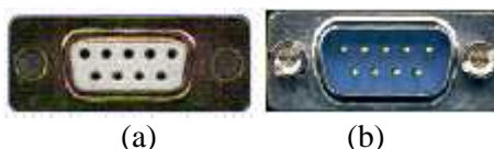
Gambar 11. (a) Konektor DB-9 Male (b) Konektor DB-9 Female [7]
