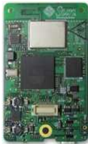
Gambar 19. Sirkuit node sensor
