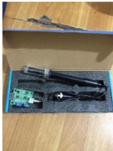
**Gambar 6.** Sensor pH Air
