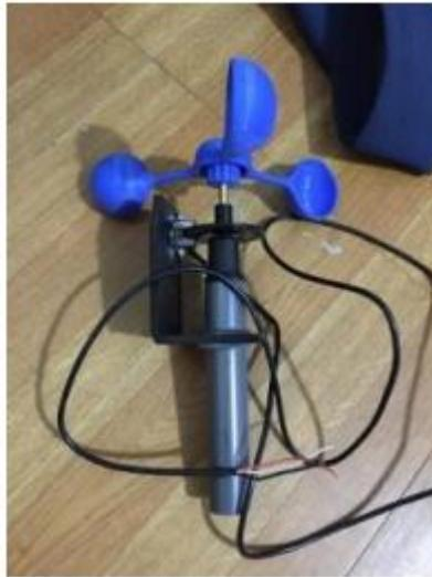
**Gambar 3.** Sensor Anemometer
