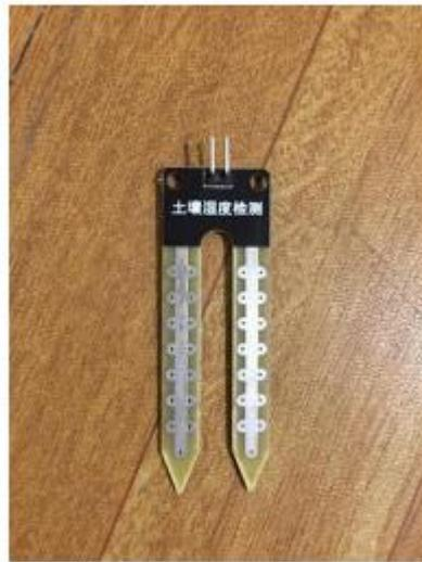
**Gambar 5.** Sensor Kelembaban Tanah
