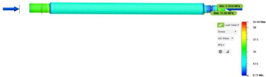
Gambar 9. Simulasi *stress* as silinder
