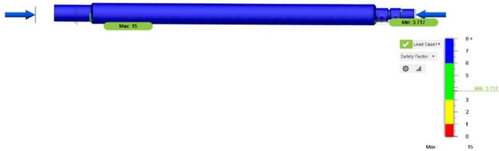
Gambar 8. Simulasi *safety factor* as silinder
