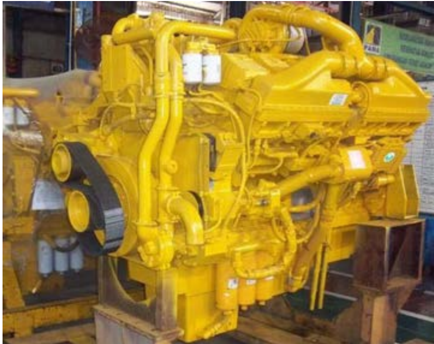
Gambar 1. Unit diesel engine cummins QSK 45
