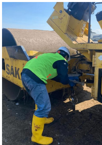
Gambar 4. Proses CBR Test Lapangan
