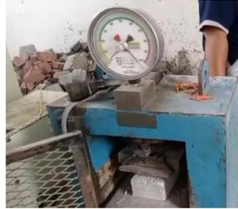
Gambar 3. Uji tekan paving block
