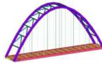
(i) Rise-span ratio =1:2,09
