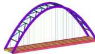
(h) Rise-span ratio = 1:2,35
