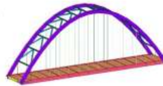
(g) Rise-span ratio = 1:2,67
