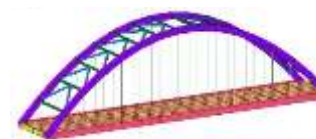
(e) Rise-span ratio = 1:3,64
