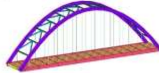
(f) Rise-span ratio = 1:3,07
