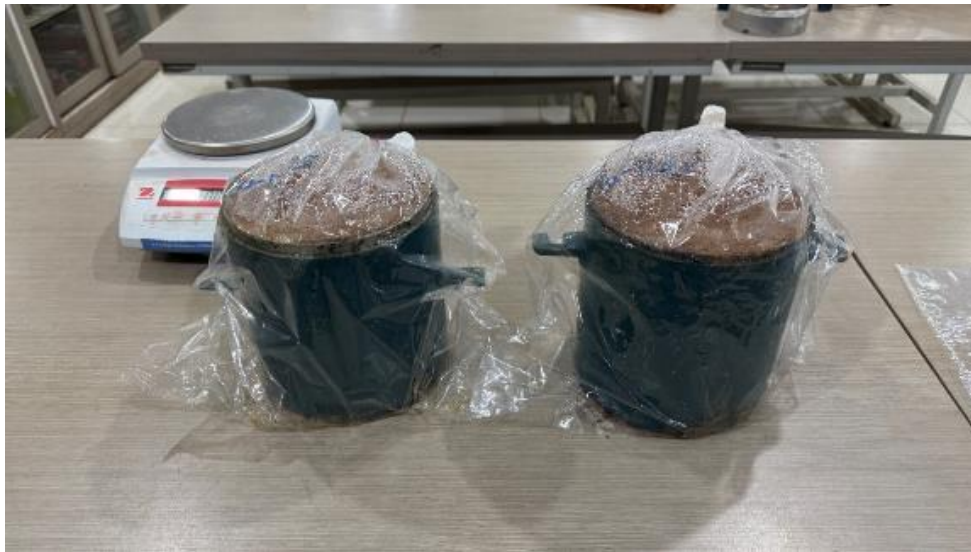
Figure 2. Samples undergoing the 14-day curing period
