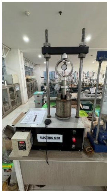
Figure 4. CBR Penetration Test Setup
