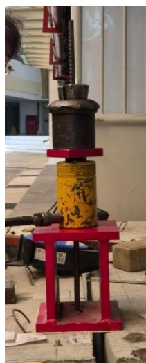
Gambar 9. Setup uji tarik angkur
