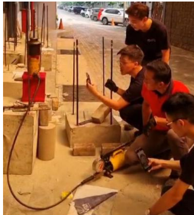
Gambar 10. Proses uji tarik ankur
