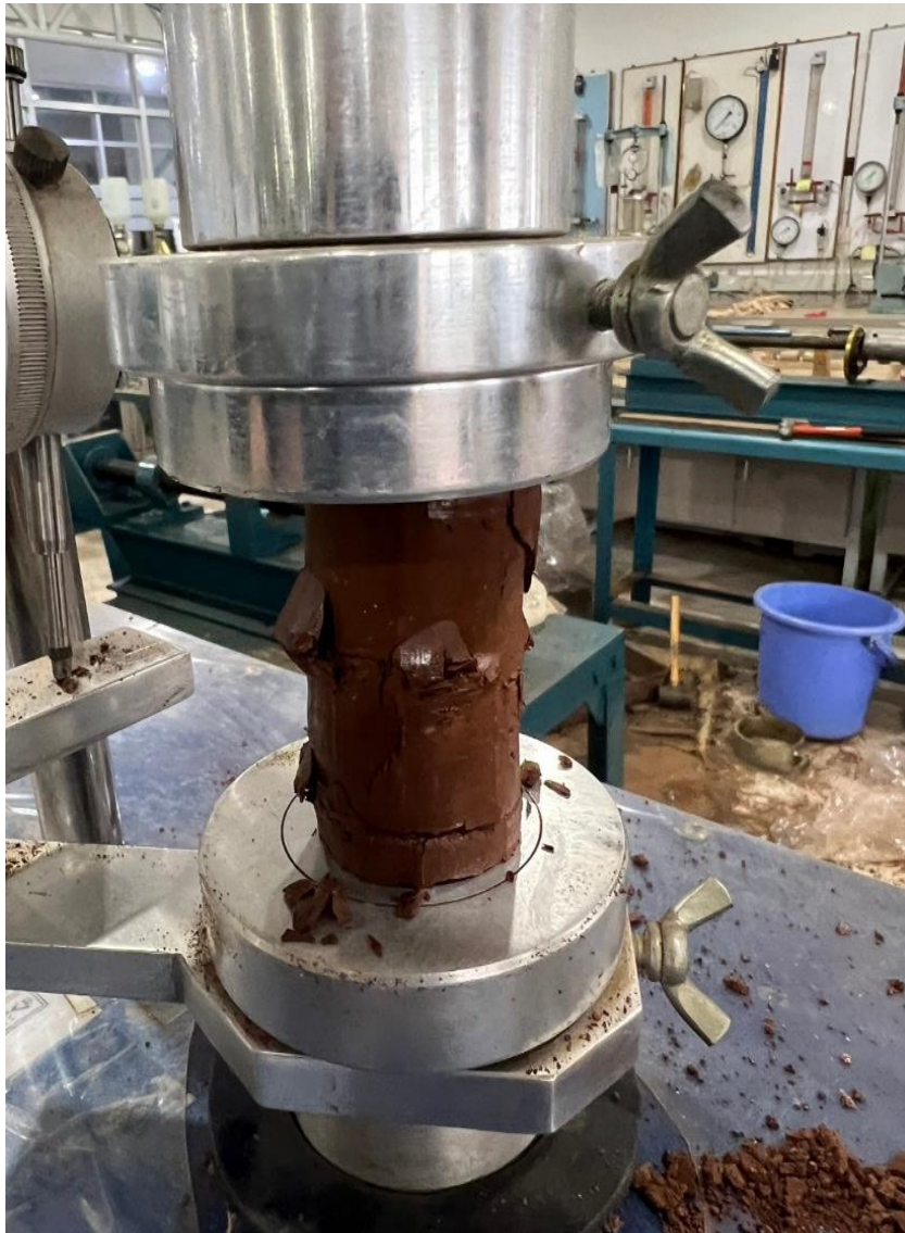
Gambar 2. Unconfined compression test
