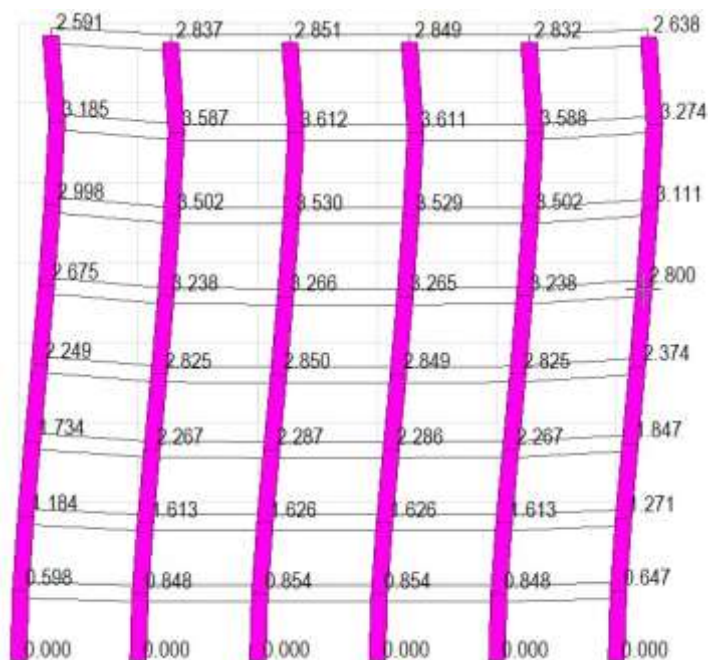
Gambar 4. Deformasi as F dengan construction stage analysis .
