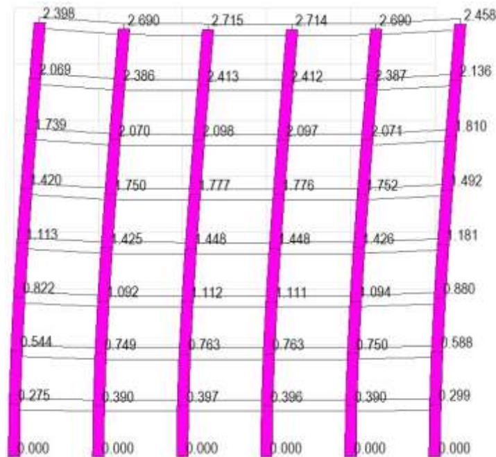
Gambar 3. Deformasi as F tanpa construction stage analysis .
