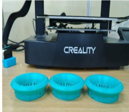
Gambar 6. Prototype Hasil Cetak 3D Funnel Air Velocity Karburator Infill Pattern Grid
