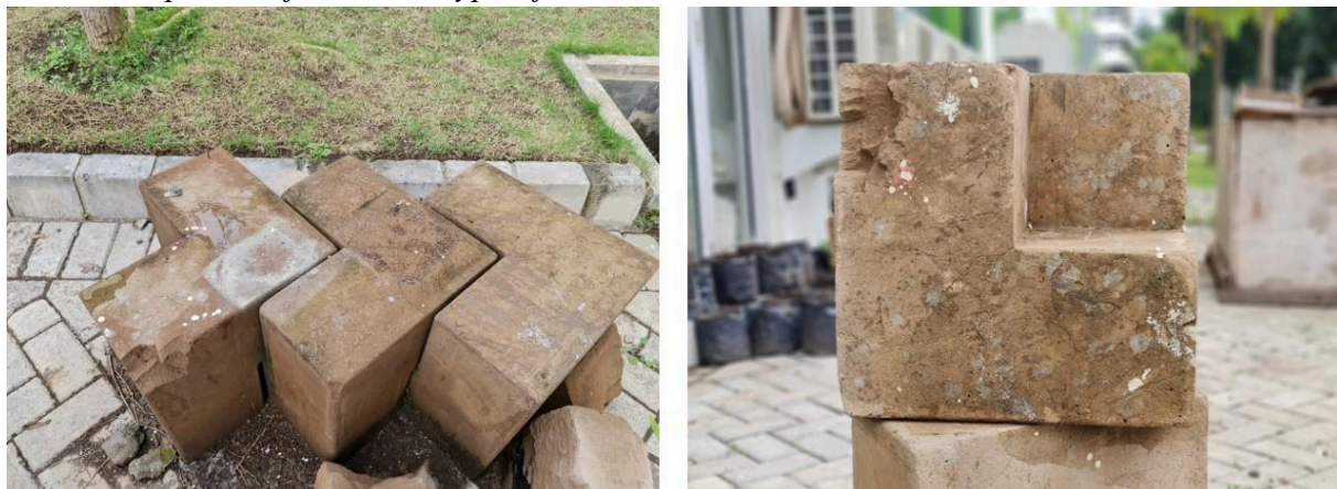
Outdoor Exposure of The Prototype After Two Years
