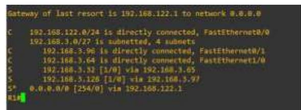
Gambar 6. Hasil Setup Static Router R1
