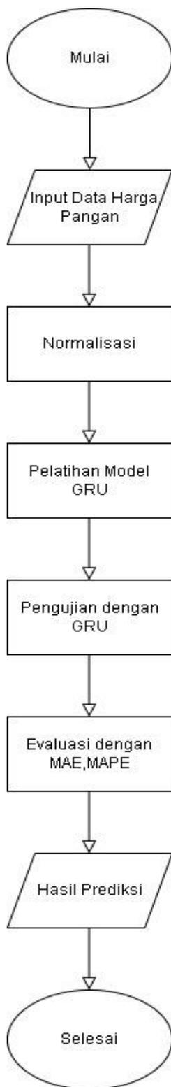
Gambar 2. Flowchar metode Gated Recurrent Unit.
