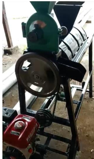
Figure 4. The Final Machine of Pellet Production
