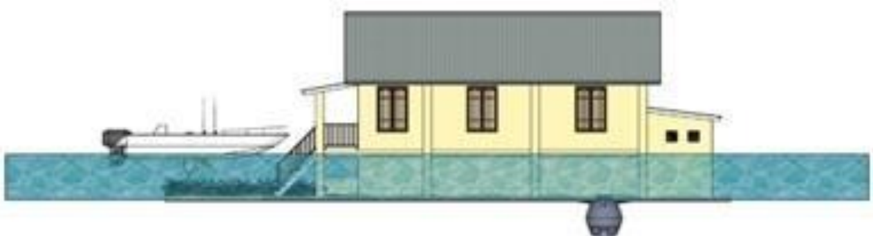
Figure 8. Simulated image of the sanitation system and evacuation conditions by canoe during a big flood Source: Authors, 2023
