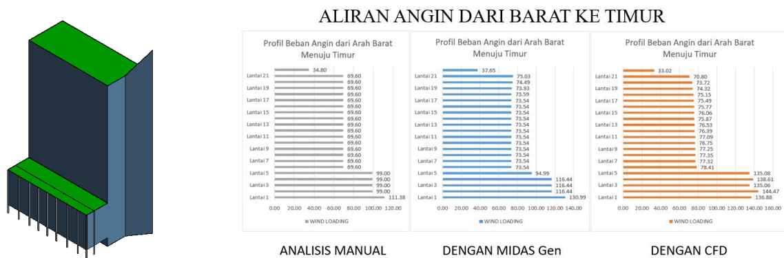
FIGURE 9 Comparative Results of Wind Load Calculation from West to East with CFD Software , MIDAS Gen, and with Manual (SNI 1727:2020)
