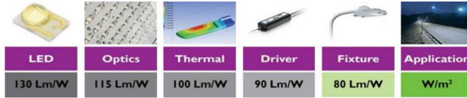
Figure 1. Luminaire Component of LED Public Street Lighting (Source: Philips)
