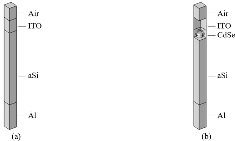
**FIGURE 3.** Amorphous silicon solar cell models (a) without CdSe QD and (b) with CdSe QD.
