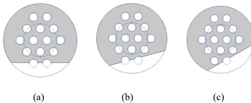
FIGURE 1. Baffles cutting angle of (a) 0°, (b) 15°, and (c) 30°
