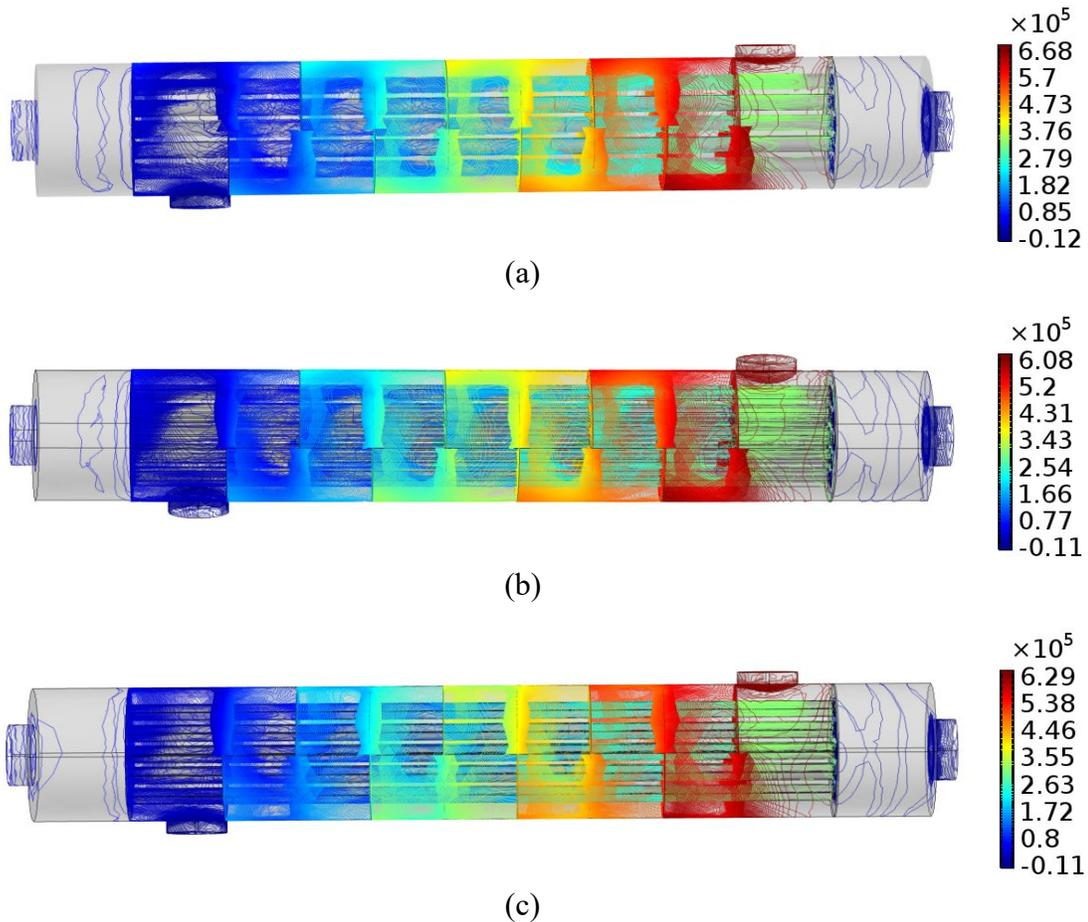
**FIGURE 7.** Pressure distribution symmetrical cut with baffle cut angle of (a)  $0^{\circ}$ , (b)  $15^{\circ}$ , and (c)  $30^{\circ}$
