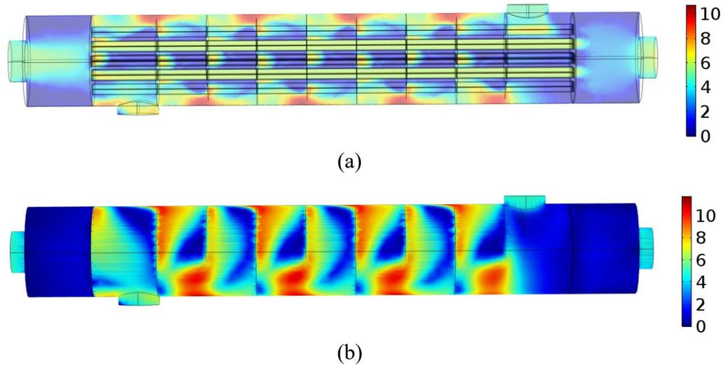
**FIGURE 6.** Velocity distribution with baffle cut angle of  $30^{\circ}$  (a) symmetrical cut, (b) full model
