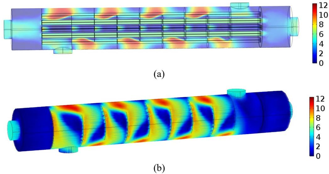
**FIGURE 4.** Velocity distribution with baffle cut angle of  $0^\circ$  (a) symmetrical cut, (b) full model
