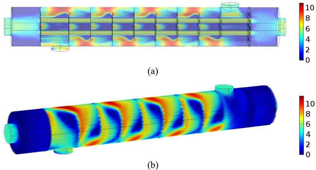
**FIGURE 5.** Velocity distribution with baffle cut angle of  $15^\circ$  (a) symmetrical cut, (b) full model
