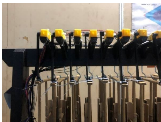
Figure 9. DC Motor on Angklung
