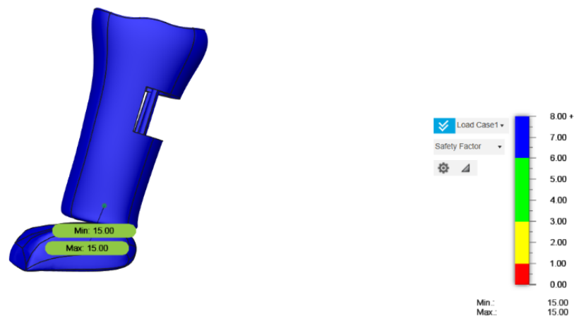
Gambar 9. Hasil simulasi Static stress – safety factor
