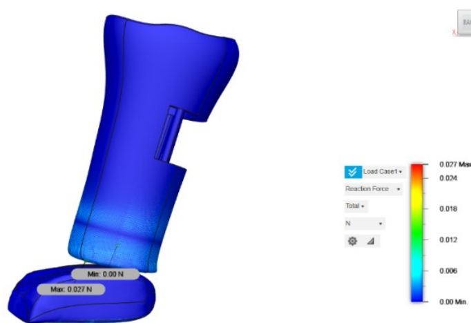
Gambar 11. Hasil simulasi Static stress – Reaction Force
